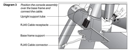
5. Position the console assembly over the base support. Diagram 3. Remove any tape that secures the RJ45 cable. Have an assistant hold the upper support tube over the base frame support (display console must face the foot pedals) while you connect the cable and align the bolt holes.
